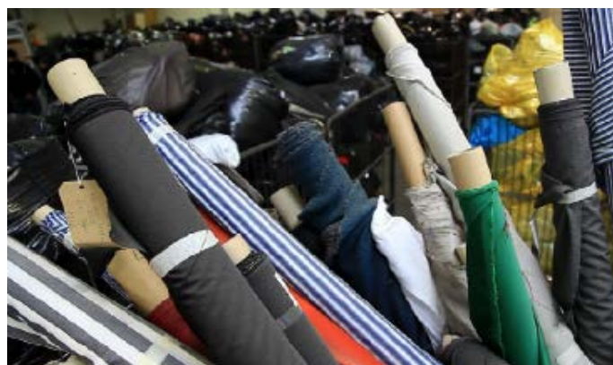
End-of-roll textile waste is factory surplus textile waste leftover on the textile rolls from garment manufacturing.
